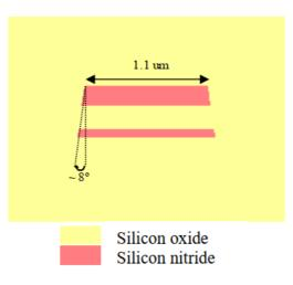
The waveguides consist of a "double-stripe" shown in TriPleX<sup>™</sup> BB using layers of Si3N4 with a high refractive index. Furthermore, the cladding and core region consist of SiO2. The complete waveguide is realized on 100 mm
