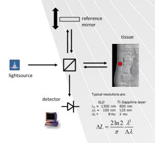
This can be implemented by either using a narrow linewidth laser which is swept in wavelength fast or a broadband lightsource where the spectral information is gathered at the detection side with a spectrum analyzer. This work deals with such a spectral domain OCT system in which a broadband lightsource is used. Schematically this is shown in the picture below.
