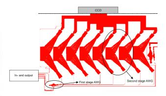
With the building blocks in the PDK a PIC was made with a cascaded Arrayed Waveguide Grating (AWG) as spectrometer and a common path interferometer was integrated on the chip as the schematic chip layout above demonstrates.
