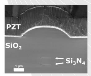
The modulator is optimized as the PZT layer geometry employs a stress-focusing behaviour on top of the waveguide stack, and at the same time allows for a thinner top cladding to further increase the stress interaction at the waveguide core and as such keeping the excess loss per modulator minimal. Using a Mach-Zehnder interferometer, we measured a half-wave voltage,  $V\pi$ , at 12 V at a wavelength of 1550 nm using a modulator with a total length of 15 mm.
