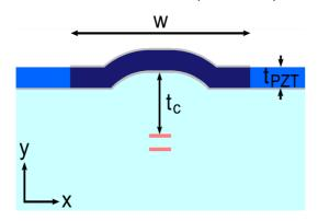
The major advantage of our stress-optic modulators over thermo-optic modulators is their ultra-low power dissipation in a static state. The static power consumption is solely determined by tiny leakage currents through the piezoelectric layer resulting in a dissipated power in the  $\mu$ W-region.
